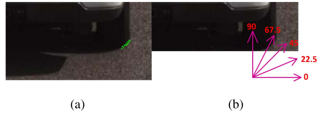
Fig. 6. (a) Detected curvature of the right tire, (b) orientation of the Gabor filter bank.
