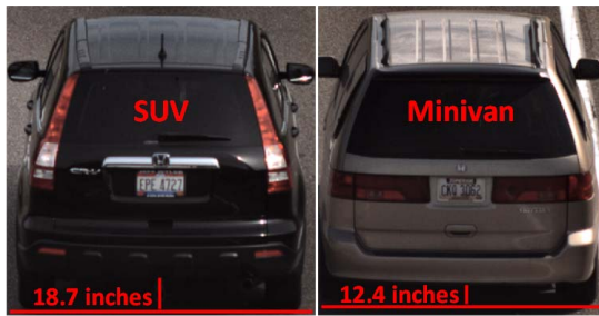
Fig. 2. Comparison of VRGC between SUV and Minivan.
